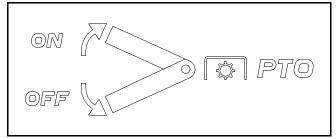
The PTO lever is located on the left side of the dashboard next to the steering wheel. Move the PTO lever forward to engage the power to the cutting deck or other (separately available) attachments; move the PTO lever rearward to disengage the power to the attachments.
